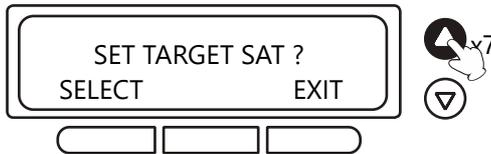
2. Press the UP button seven times to enter set GPS.
