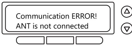
1. Check the RF cable between the antenna and the ACU
