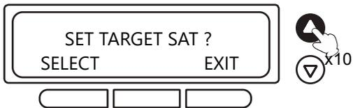
2. Press the UP button ten times to enter antenna move step.
