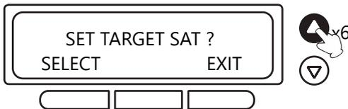
2. Press the UP button six times to enter set parameters.
