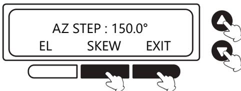
4. Input position value for azimuth axis.
